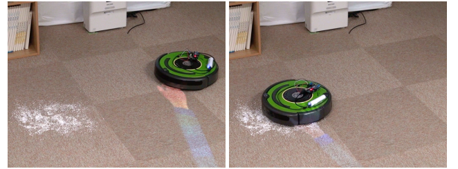
Figure 11: Cleaning robot manipulation: (left) the closing gesture grabbed the robot, and (right) the opening gesture released it at the place to be cleaned up.
