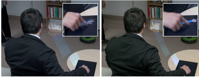
Figure 15: Tremor suppression technique: (left) without and (right) with stabilization technique. Three captured frames are overlaid and blended to show the tremor effects .
