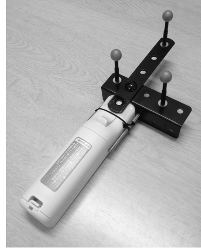
Fig. 4. Hand held device attached by three MoCap markers.
