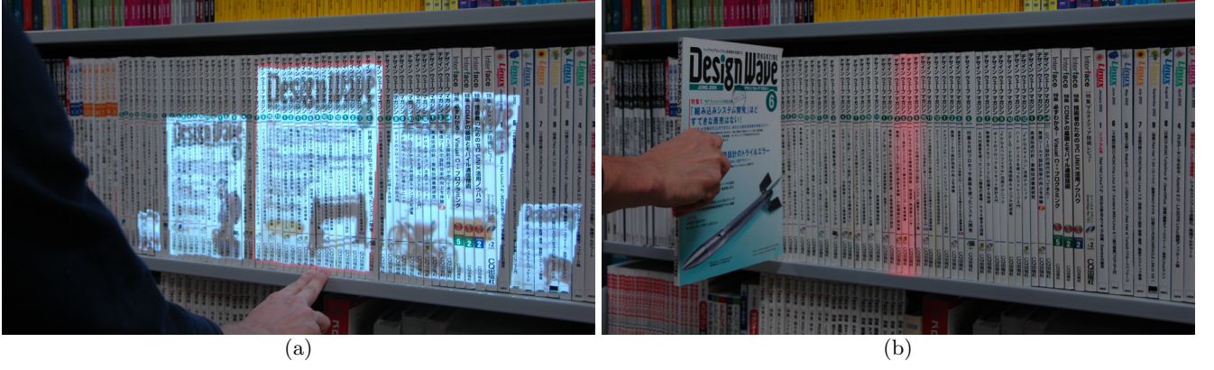
Figure 1: Proposed in situ book searching and storing support: (a) book searching support by projecting the cover image of a stored book onto the spines, (b) book storing support, in which when a user brings a book close to the bookshelf, a spotlight is projected onto the place where the book should be stored.
